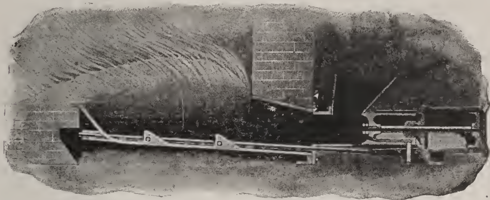
FIG. 108. SECTIONAL VIEW OF JONES UNDER-FEED STOKER.
